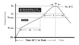
Infrared Reflow: 260°C, 30 seconds max.
