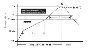
Wave Soldering: 260°C, 10 seconds max. Infrared Reflow: 260°C, 30 seconds max.
